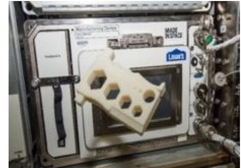
Additive Manufacturing Facility (AMF) on ISS developed via SBIRs with Made in Space, Inc.
