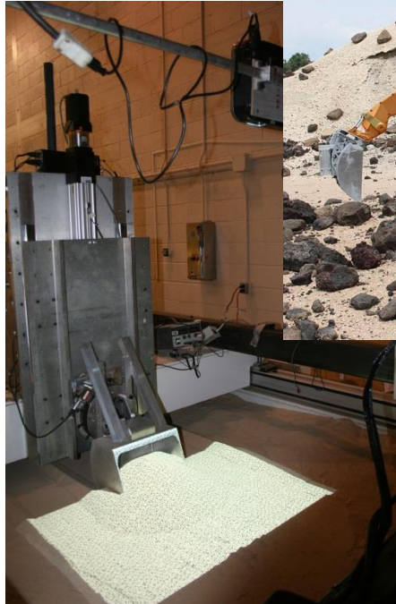
Excavation force determination with soil surface 3D measurement using structured light stereography
