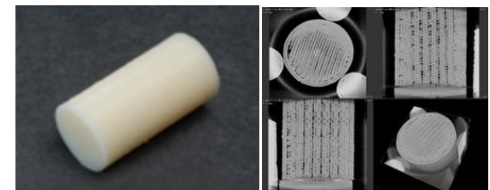
CT Scan (right) of compression cylinder manufactured on ISS (left).
