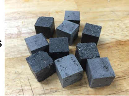
Standard 2-inch cube compression test specimens
