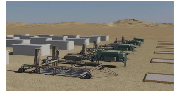
3D print 32' x 16' x 8' barracks with locally sourced concrete, within 48 hrs of deployment
