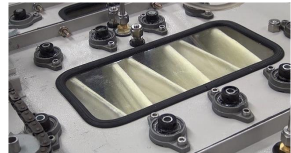
Scroll filter designed for Space Station
